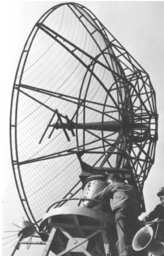
A radar mast, which could track enemy ships and planes, is adjusted on a U.S. Navy ship in 1945.
